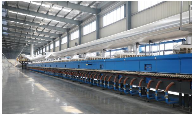
拥有428组火焰烧嘴，长（260米）辊道窑 With 428 groups of flame burner, domestic the longest (260 meters) roller kiln
